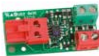
BUS XIB interface (for E045 or E024S control unit with non BUS photocell)
